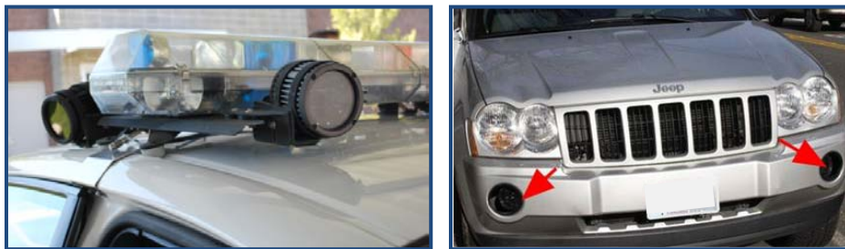
Figure 6: Lightbar (left) and Covert (right) Mounted Mobile ALPR Cameras
