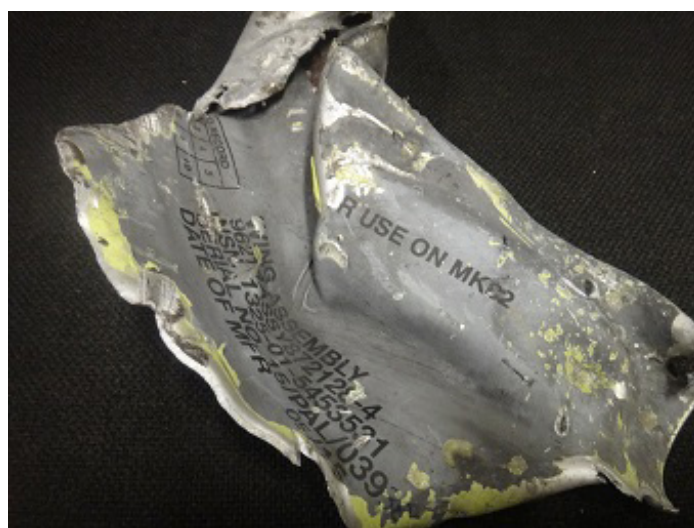
Remnant of a UK-made Paveway IV bomb found at the scene of the attack on Al-Muqbeli Warehouse. As the marking “FOR USE ON MK-82” indicates, a US-made Mk-82 warhead was used with the Paveway IV bomb. The marking “NSN1325-01-545351” is associated with the Paveway IV wing assembly. The marking “96214” identifies Raytheon as the manufacturer, and the marking “05/15” identifies the weapon’s date of manufacture as May 2015.
