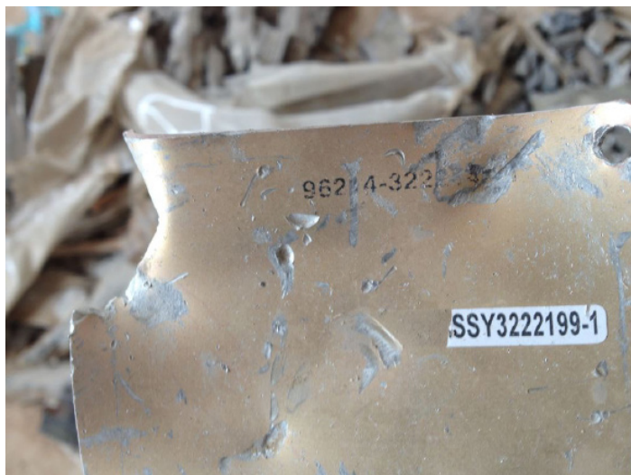
A remnant of a large guided bomb unit recovered at the scene of an attack on a civilian home in Amanat Al-Asimah Governorate (see Section II). The marking “96214” identifies US defense contractor Raytheon as the manufacturer.
