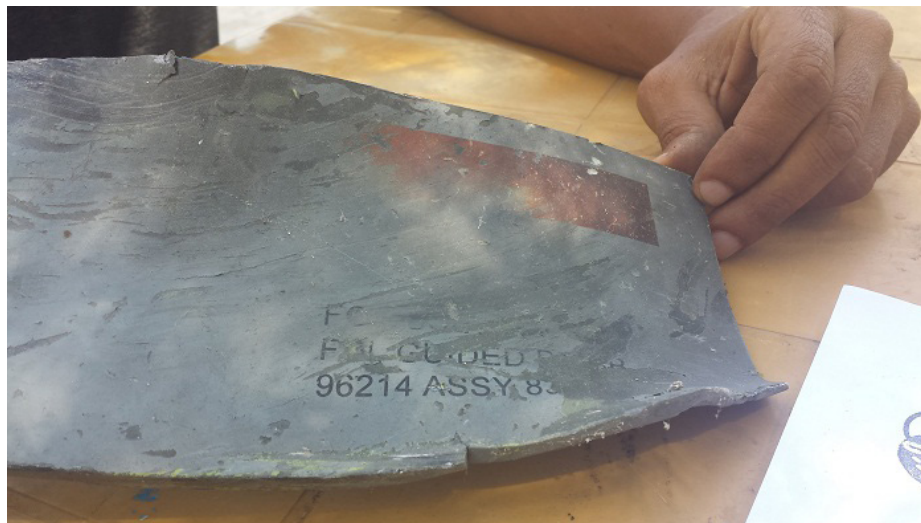
Remnant of a Raytheon-manufactured guided bomb unit recovered at the scene of the attack on the Cultural Center. The marking “96214” refers to US defense contractor Raytheon’s CAGE number.
