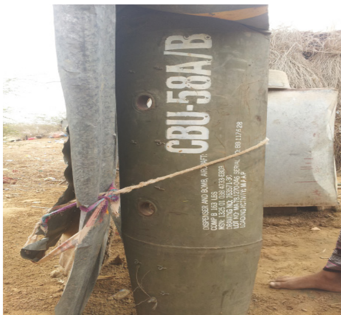
A US-made CBU-58 cluster bomb casing recovered at the scene of the attack in Bani Haddad village. The CBU-58 cluster bomb disperses about 650 BLU-63 submunitions widely and indiscriminately.
