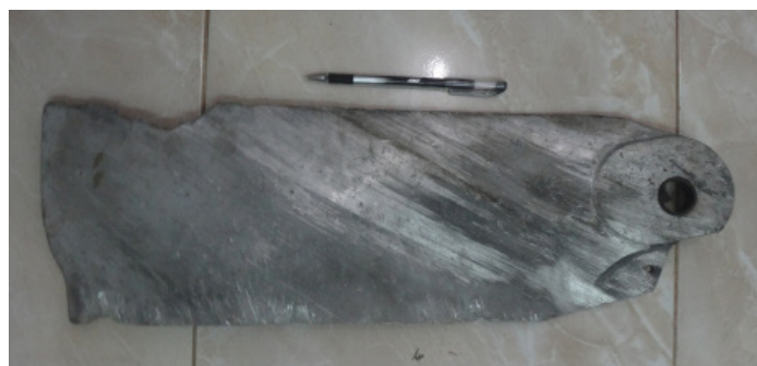
Remnants of a US-made GBU-12 Paveway II bomb recovered at the scene of the attack that killed Haifa Zawqari. As the marking “FOR USE ON MK82” indicates, an Mk-82 warhead was mounted on the GBU-12 bomb. The marking “1325-01-041-5890,” parts of which are visible in the photo on the left, is associated with a Raytheon-manufactured wing assembly.
