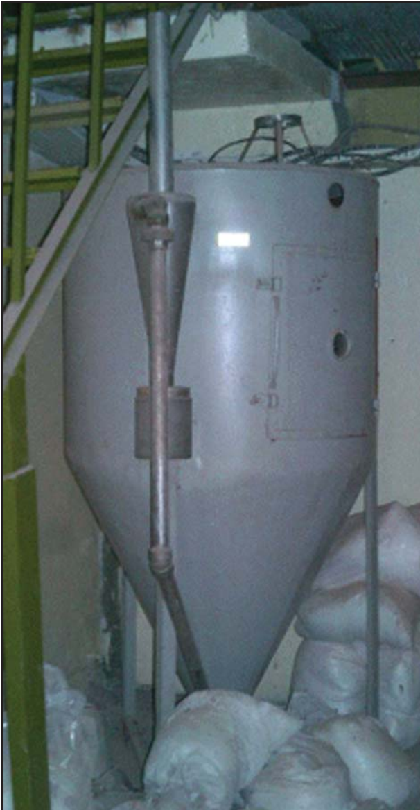
Figure 7. Example of dual-use biological processing equipment found at TABRC (spray dryer).
