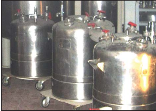
Figure 13. 1m 3 Stainless steel mobile tanks.
