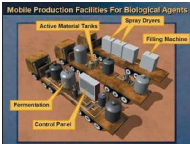
Figure 11. Truck-mounted BW production unit—based on source reporting.
