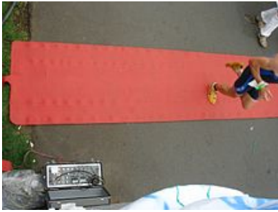
J-Chip 8-channel receiver next to timing mat. The athlete wears a chip on a strap around his ankle. Ironman Germany ( https://web.archive.org/web/19961218232821/http://www.ironman.de/ ) 2007 in Frankfurt.
