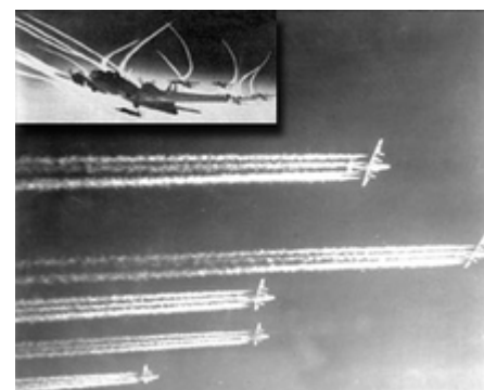
Contrails from propeller-driven aircraft engine exhaust, early 1940s
