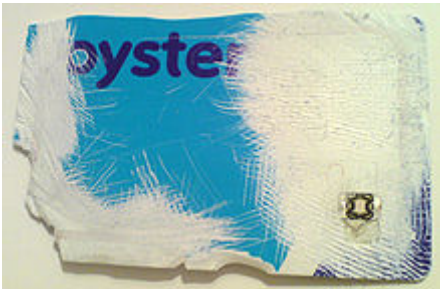
An RFID tag, exposed by the damage to this Oyster card
