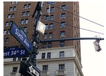
RFID E-ZPass reader attached to the pole and mast arm (right) used in traffic monitoring in New York City
