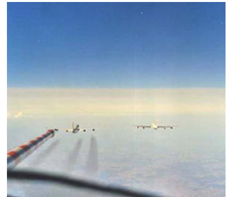
Contrail testing being carried out on an Airbus A340 and much older Boeing 707 [6]
