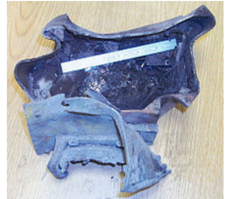
The cockpit voice recorder from Flight 77 was heavily damaged from the impact and resulting fire.
