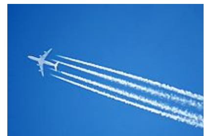
A high-flying jet's engines leaving a condensation trail ( contrail )
